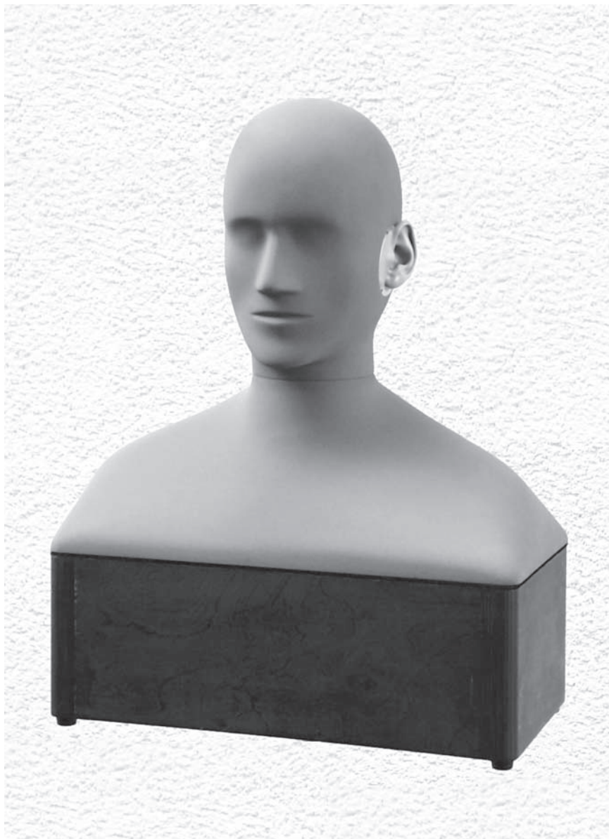
Figure 7.1 Dummy head (Institute of Technical Acoustics, Aachen, Germany).
