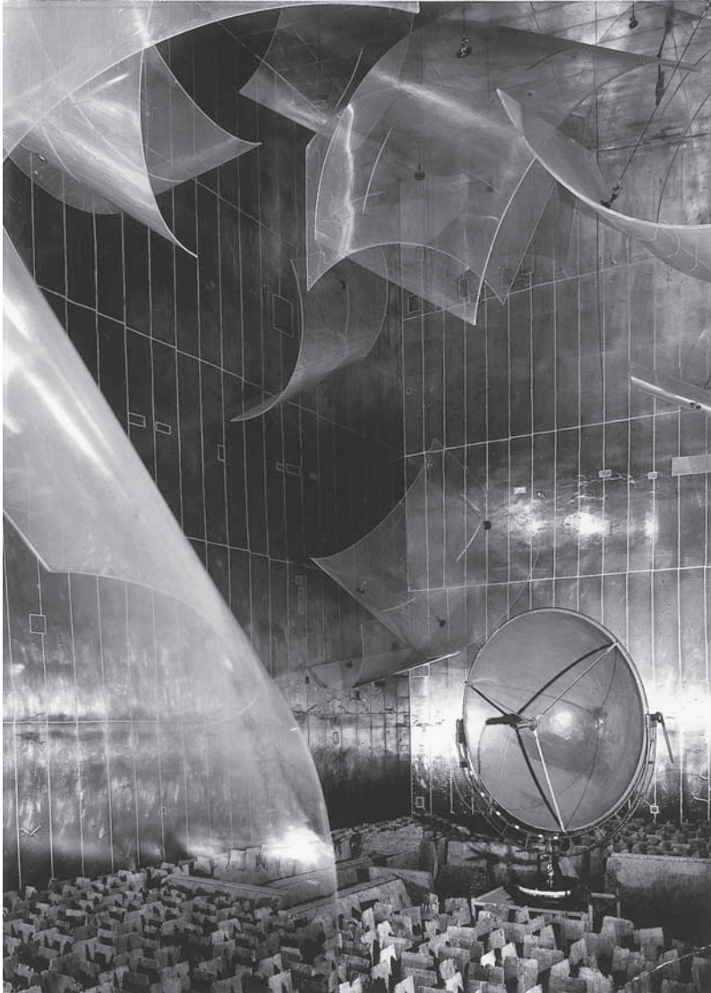
Figure 8.18 Reverberation chamber fitted out with 25 diffusers of perspex (volume 324 \text{ m}^3 ; dimensions of one shell 1.54 \text{ m} \times 1.28 \text{ m} ).
