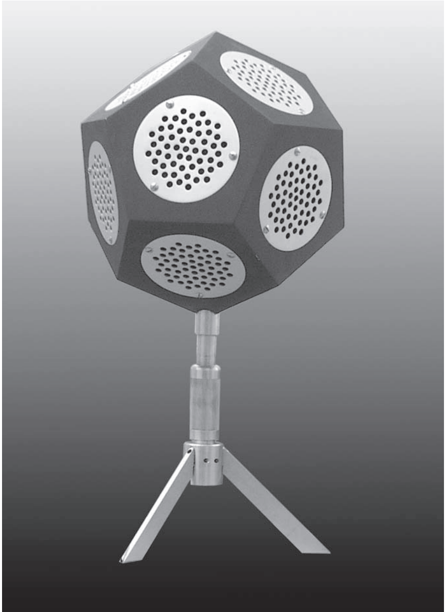
Figure 8.1 Dodecahedron loudspeaker for acoustical measurements.
